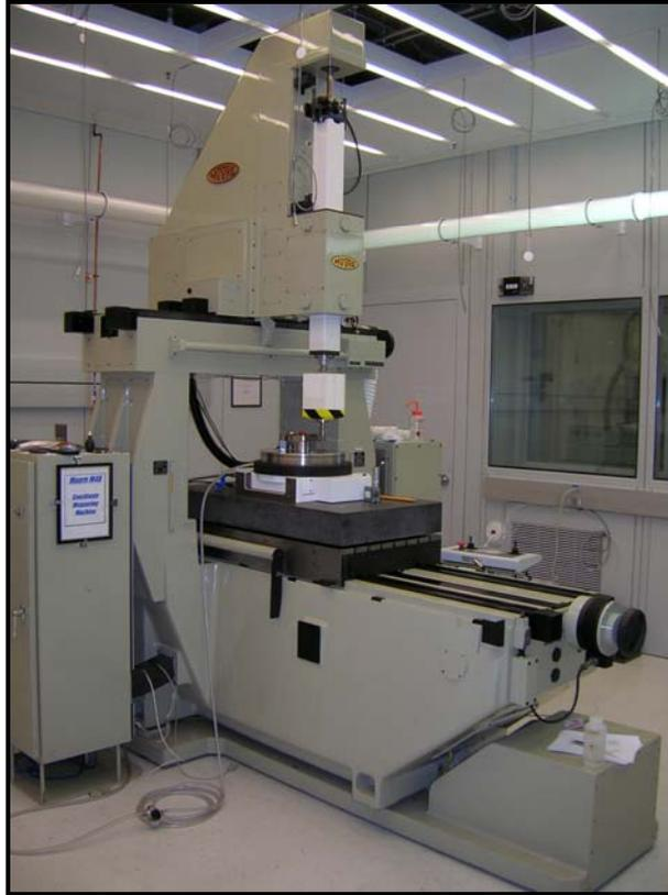
Figure 1. The NIST M48 coordinate measuring machine in the Advanced Measurement Laboratory.
