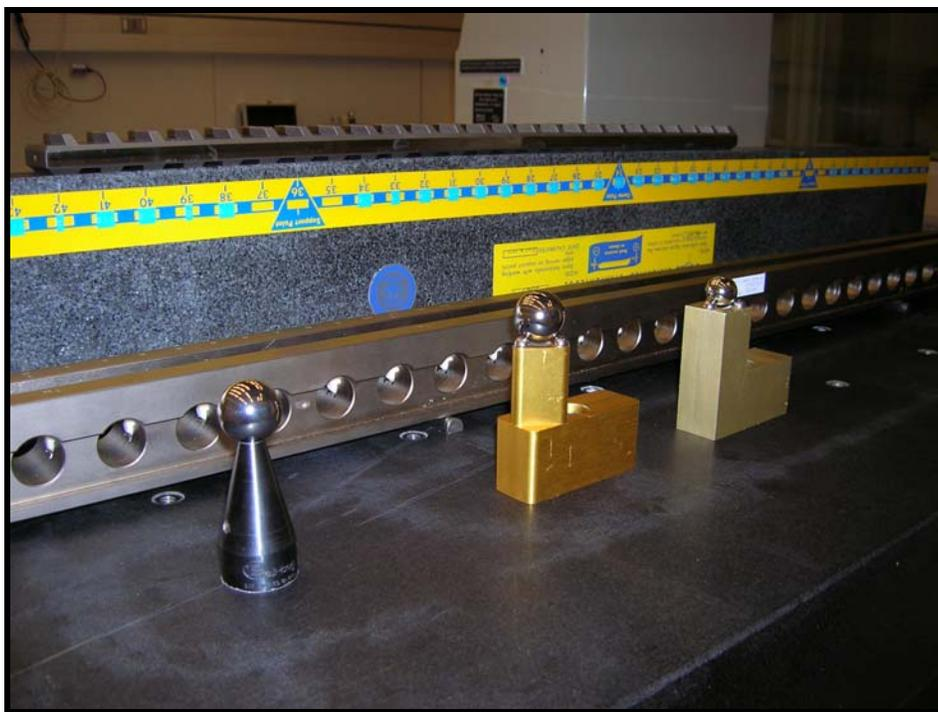
Figure 7. CMM calibration sphere and precision stainless steel master spheres, in magnetic kinematic mounts, on the CMM table.
