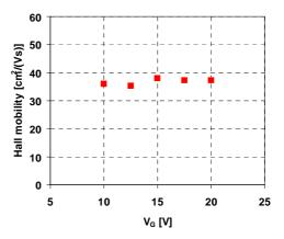
Fig. 6. Hall mobility calculated from  $R_s$  and  $n_s$  as a function of gate voltage.
