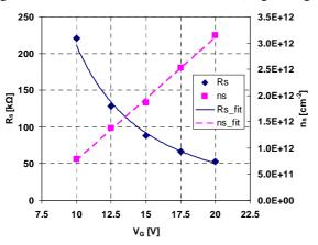
Fig. 5. Sheet resistance and inversion sheet charge density measured at different gate voltages.
