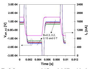
Fig. 3. Source current and AC coupled differential voltage corresponding to the drain voltage modulation. Four magnetic fields are used. As B increases, dV<sub>diff</sub> gets larger.
