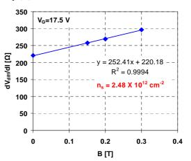
Fig. 4. Inversion sheet charge density ( $n_s$ ) extraction at  $V_G$ =17.5 V.
