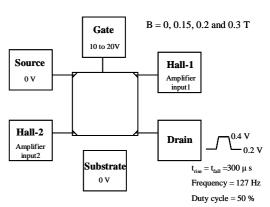
Fig. 2. The 4H-SiC Van der Pauw structure measured, which has an active gate area of 150  $\mu$ m  $\times$  150  $\mu$ m. The setup shown here is for the inversion sheet charge density (n<sub>s</sub>) measurement.
