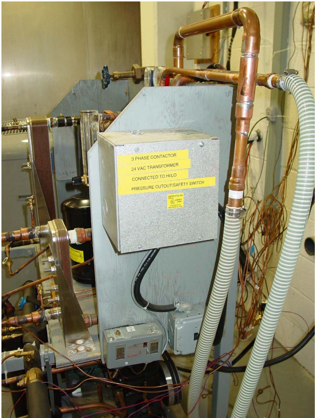
Figure B5: Right side view of water cooled condensing unit showing power contactor box, hi/lo pressure safety switch, and manual on/off switch
