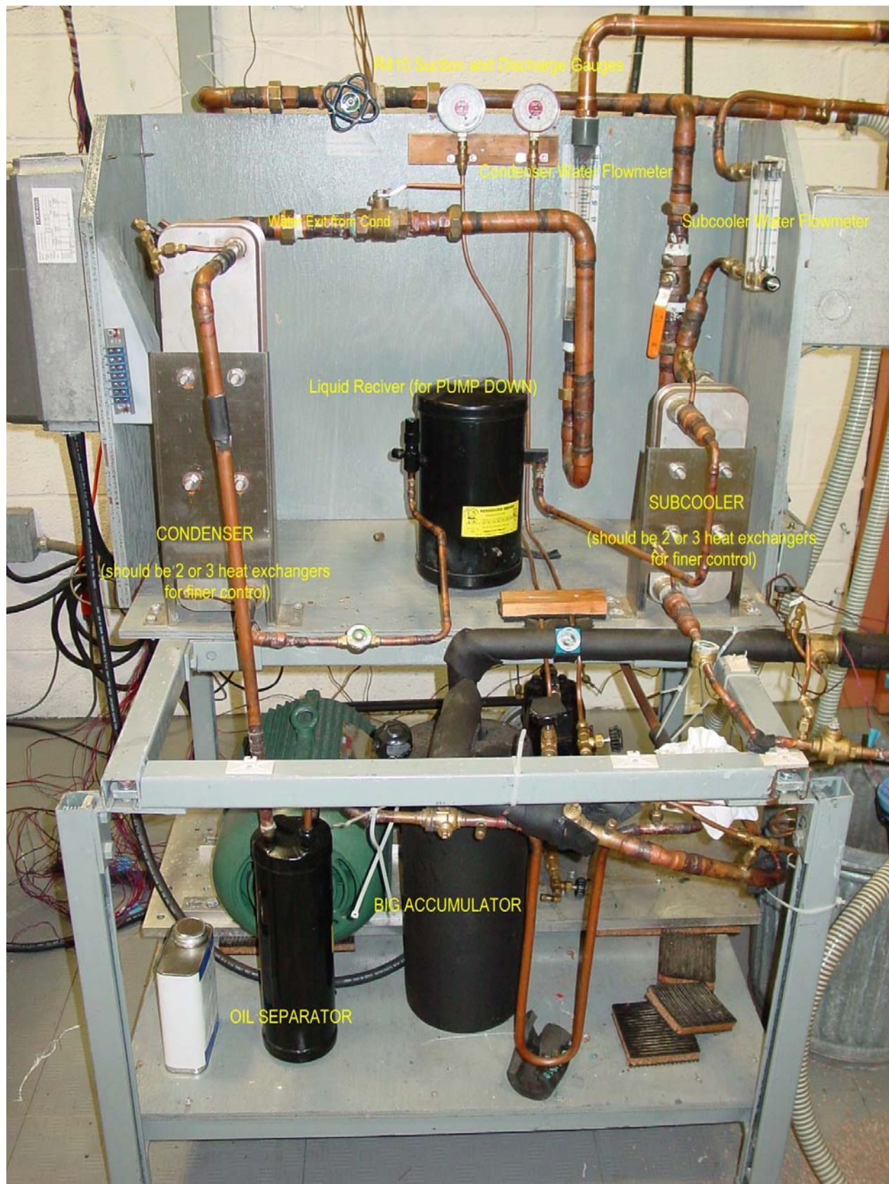
Figure B1: Water-cooled condensing unit with variable-speed, open-drive compressor
