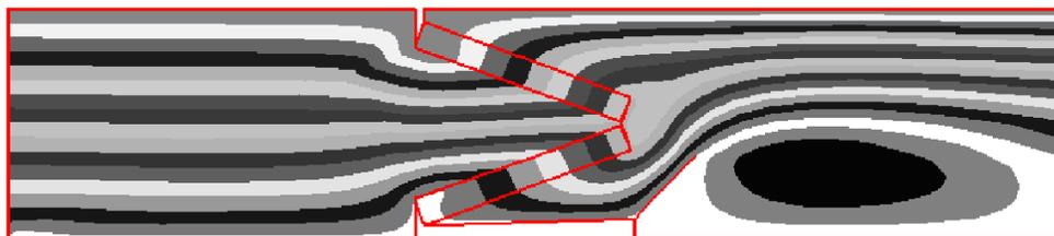
Figure 4 Streamlines for Flow through Dry Coil at 1200 CFM
