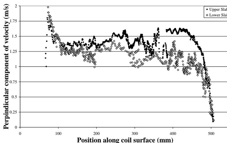
Figure 3 Air Velocity Profiles for Inlet to Dry Coil at 1200 CFM
