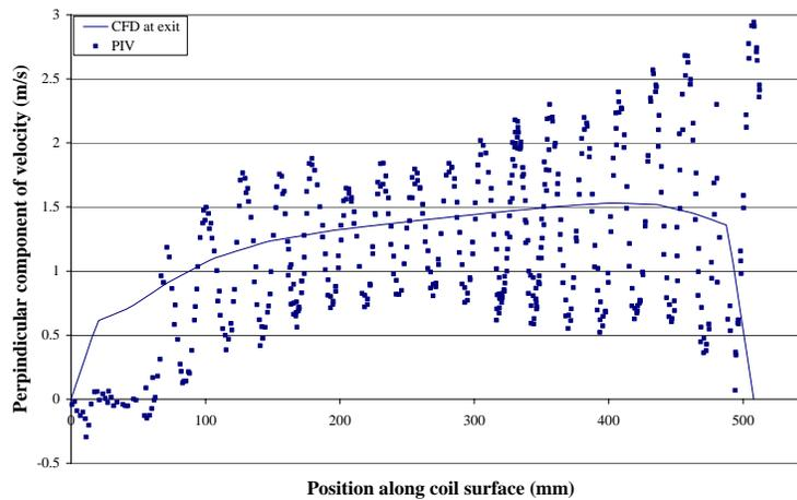
Figure 5 Measured and Predicted Air Velocity Profile for Exit from Top Slab of Dry Coil at 1200 CFM
