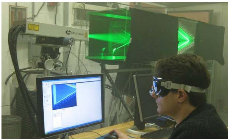
Figure 2 PIV Data Collection for Inlet Air Velocity Profile
