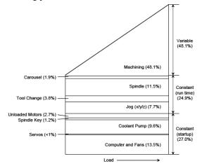
Figure 4. Energy consumption of a machining system (adopted from [21])
