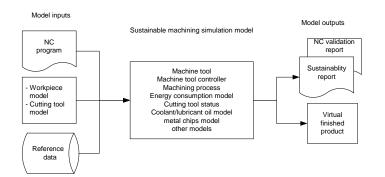
Figure 3. Proposed virtual machining model with environmental impacts analysis
