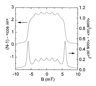
FIG. 4. Approximate analytic results, Eqs. (2) and (3), for  $(N - 1) - \langle \cos \delta \theta \rangle$  (the theory equivalent of the magnetoresistance) and it variance for a 7-layer system with  $mB_1/J_{\perp}=2.5$  and  $k_BT/J_{\perp}=0.3$ , roughly the conditions realized experimentally in the case of the 7-layer sample in Fig. 1(b), (assumes that  $m=2 \times 10^6 \mu_B$ ). Monte Carlo results obtained for Eq. (1) are nearly indistinguishable from the solid lines.
