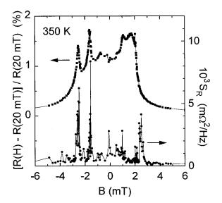
FIG. 2. Plot of magnetoresistance and resistance noise power spectral density at 1 Hz for a 7-layer, 16- $\mu$ m wide, 160- $\mu$ m long device at 0.8×10<sup>7</sup> A/cm<sup>2</sup> and at 350 K. *R* (20 mT)≈30.9  $\Omega$ . The plot shows the strong correlation between regions of high noise and peaks in the magnetoresistance.
