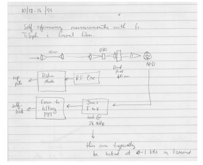
**Figure 2**: (a) Lab book diagram of the initial scheme for measuring and stabilizing  $f_0$ . A split tube piezo transducer in the linear cavity of the femtosecond laser could be driven in two different modes. The piston mode was used to lock the laser repetition rate, while the tilting mode was used to stabilize  $f_0$ . The ideas and hardware for the split piezo and its high voltage driver, the avalanche photodiode (APD), and frequency to voltage converter (F to V) all came from Jan
