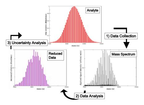
Figure 1— Steps of a complete measurement: data collection, data analysis, and uncertainty analysis.
