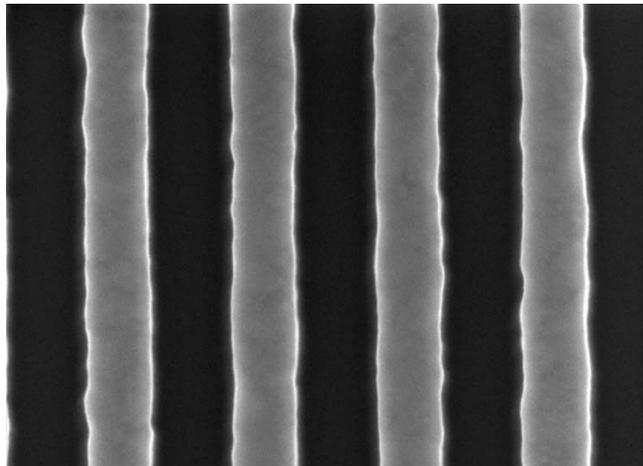
Figure 8. Typical SEM image of the 200 nm pitch patterns at 100 000 times magnification.
