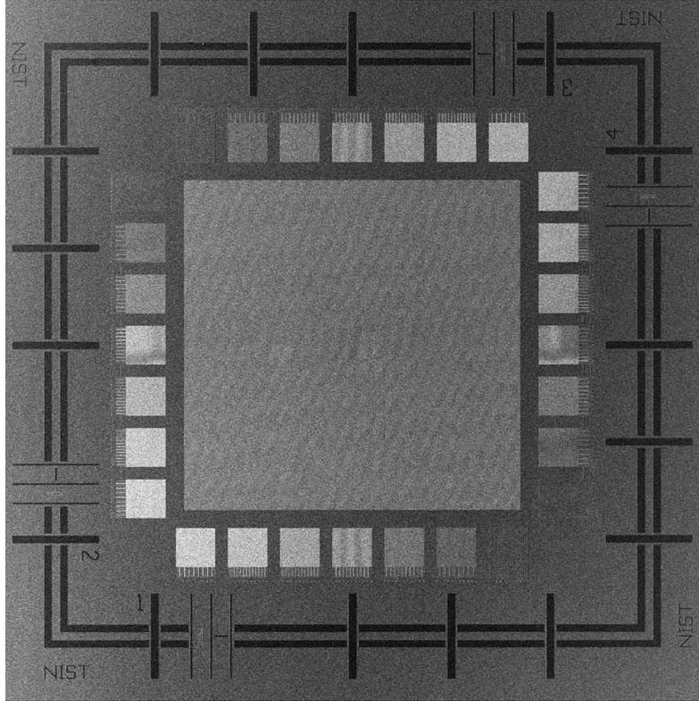
Figure 6. SEM micrograph of the whole RM 8820 structure. The pitch values of the large square frame structure are 1.5 mm in both X and Y directions as shown in Figure 4.
