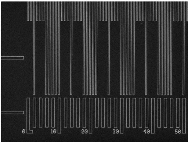
Figure 7. Typical low-magnification image of a roughly 50  $\mu\text{m}$  portion of the binary-type pitch structure. The 2  $\mu\text{m}$  pitch-numbered guiding lines at the bottom and the isolated and dense structures are clearly visible.
