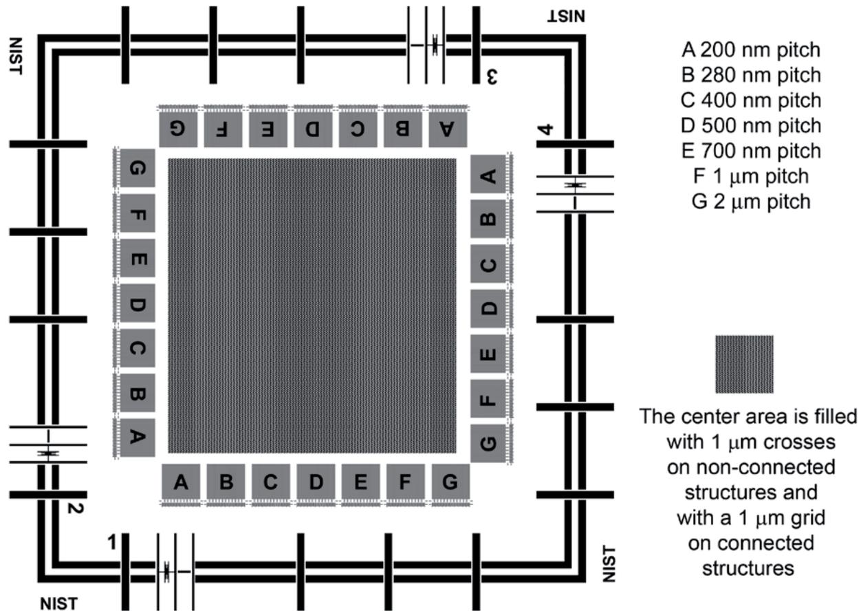
Figure 5. The nominal X and Y direction pitch values for the small A to G structures of RM 8820.
