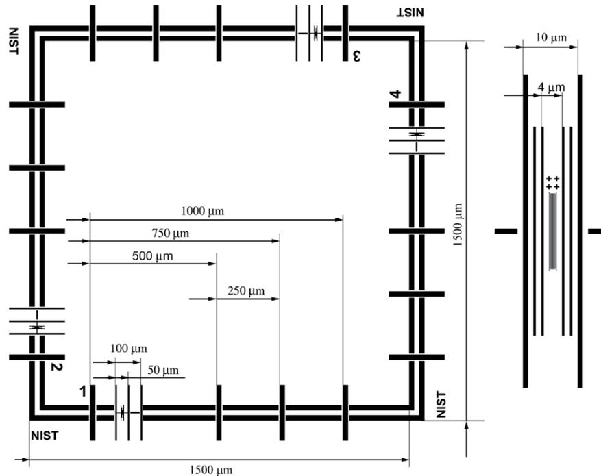
**Figure 4. The nominal X and Y direction pitch values for the large structures of RM 8820.**
