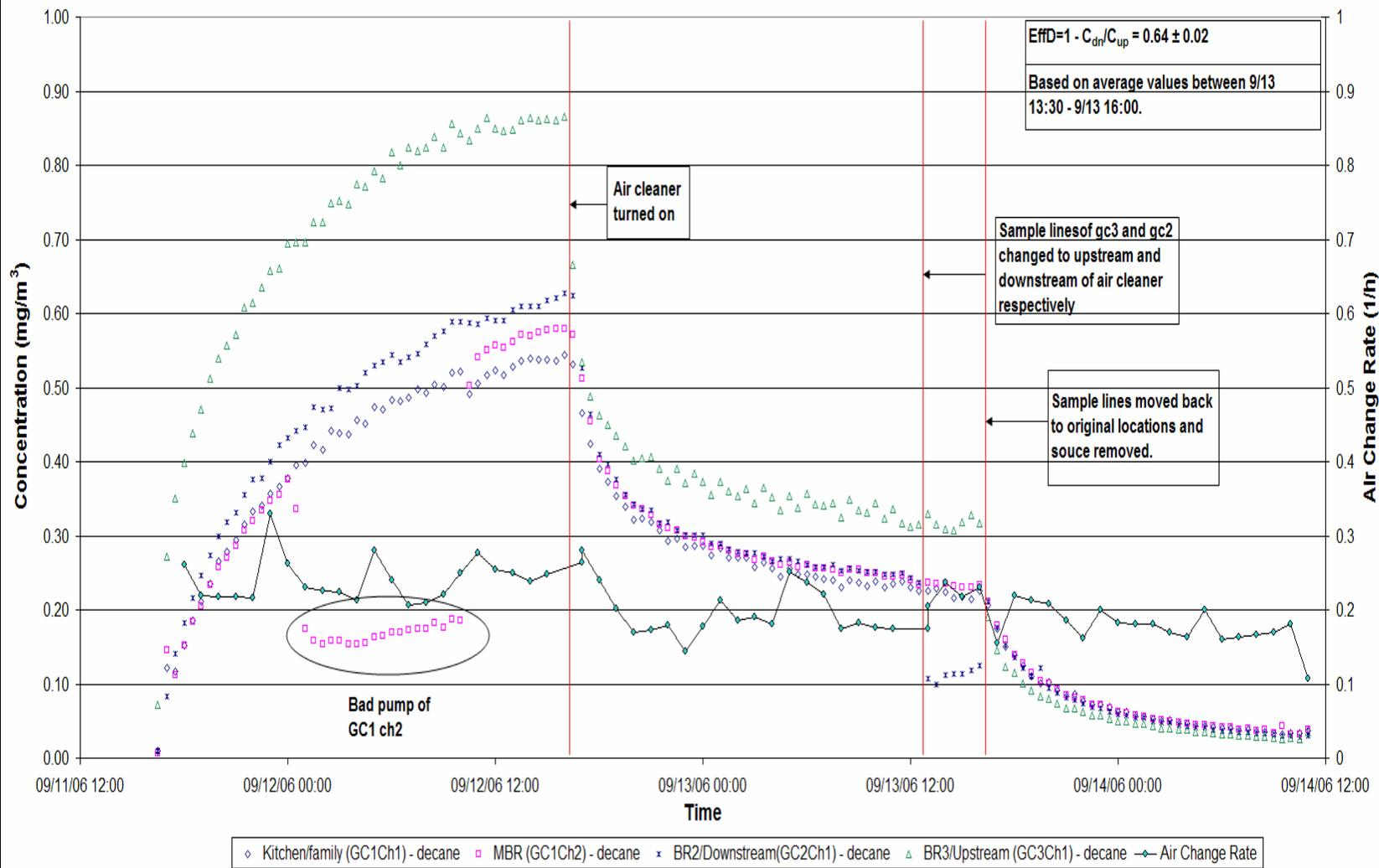
**Figure 4: Test #53/PAC - Decane injected in BR3; all mix fans off; HVAC off; BR3 door closed, all other doors open; Portable air cleaner installed in BR3.**
