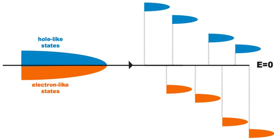
Figure 1: Schematic of the eight-fold symmetry breaking of the zero energy Landau level in graphene bilayers. Vertical axis is energy, while offsets in the horizontal axis are done for visual clarity.
