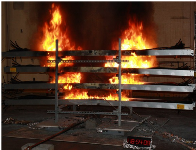
FIGURE 14. Photograph of a multiple tray test involving a thermoplastic cable.
