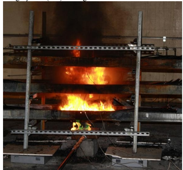
FIGURE 12. Photograph of a multiple tray test involving a thermoset cable.
