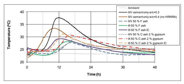
FIGURE 7 Measured semi-adiabatic temperature vs. time for HVFA mortar mixtures.
