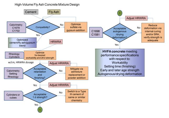
FIGURE 1 Proposed Mixture Proportioning Methodology for HVFA Concretes.
