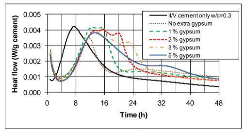
FIGURE 3 Isothermal calorimetry results normalized per gram of cement for Type II/V cement - class C fly ash (50:50) pastes with various addition levels of gypsum.
