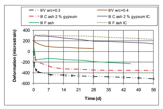
FIGURE 6 Measured autogenous deformation for sealed mortar specimens. Error bars (one standard deviation between three specimens) are provided for the II/V w/c=0.3 data to provide an indication of variability.
