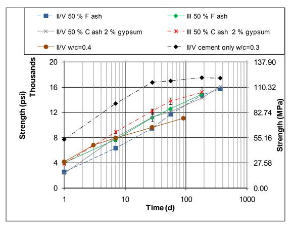
FIGURE 5 Measured mortar cube compressive strengths. Error bars (one standard deviation between three specimens) are provided for the Class C ash – III 2 % gypsum data to provide an indication of variability.
