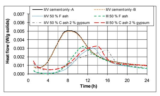
FIGURE 4 Isothermal calorimetry results normalized per gram of binder for mortars with and without 50 % fly ash. Two replicates are shown for the cement-only mortar to provide an indication of variability in the technique.
