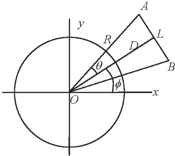
Fig. 1. Reference  $AB$  of length  $L$  positioned distance  $D$  from the tracker located at  $O$ . The range to the targets at  $A$  and  $B$  is  $R$ . The reference length  $L$  subtends an angle  $2\theta$  at the origin  $O$  and the bisector of  $L$  is located at an angle  $\phi$  from the  $x$  axis.
