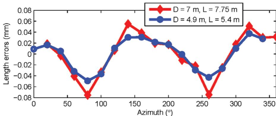
**Fig. 6.** Length errors (residuals from the mean length) are shown in the figure for horizontal length tests for two different combinations ( $D = 7 \text{ m}$ ,  $L = 7.75 \text{ m}$  and  $D = 4.9 \text{ m}$ ,  $L = 5.4 \text{ m}$ ) with azimuths taken from the original encoder map of the tracker (i.e., before correcting the tracker map for second order errors). Data was collected from tracker A.
