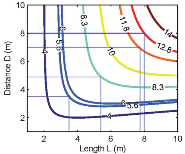
Fig. 4. Contour plot showing sensitivity (function value  $f$  in units of micrometers of length error per one microradian of second harmonic in the scale error) as a function of  $D$  and  $L$ .
