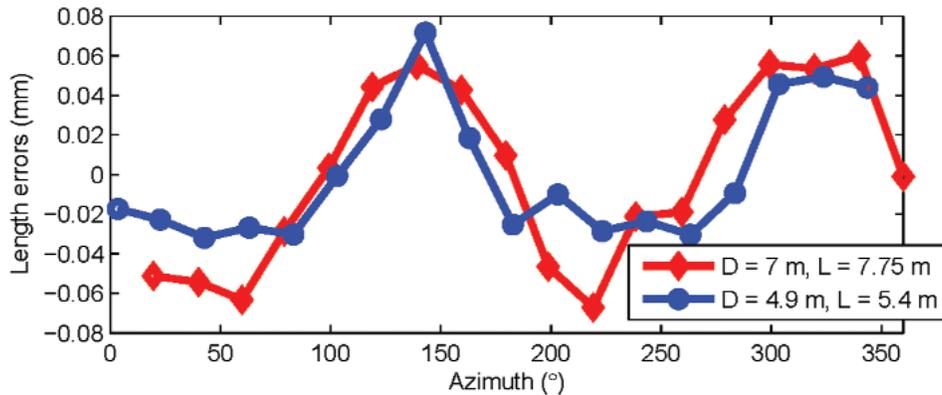
Fig. 9. Length errors (residuals from the mean length) are shown in the figure for horizontal length tests for two different combinations ( $D = 7$  m,  $L = 7.75$  m and  $D = 4.9$  m,  $L = 5.4$  m) with the original encoder map of the tracker (i.e., before correcting the tracker map for second order errors). Data was collected from tracker C.
