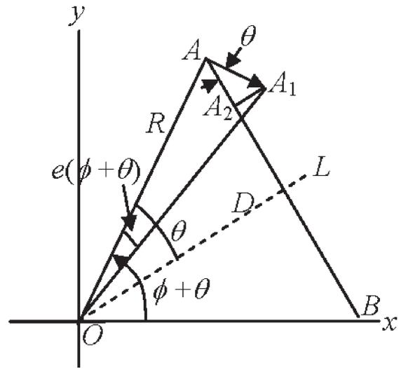
Fig. 2. Calculating the error in the length  $AB$  due to scale error in the encoder.
