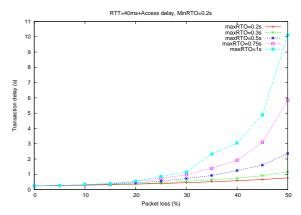
Fig. 3 Delays to transmit an indication using TCP as transport protocol
