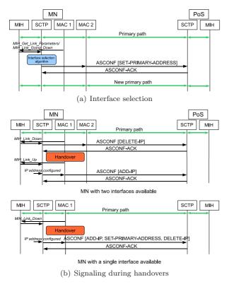
Fig. 6 SCTP signaling using MIH Services
