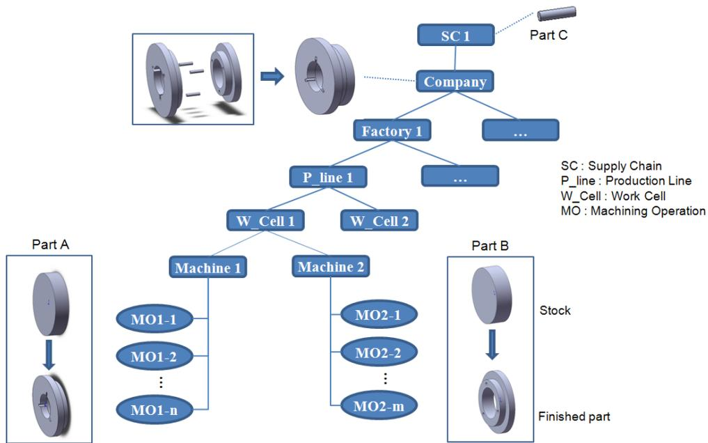
Figure 5. Manufacturing process of the selected subassembly example
