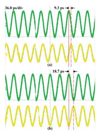
**Figure 4** Measured 90° and 180° phase shifting. [Color figure can be viewed in the online issue, which is available at wileyonlinelibrary.com]
