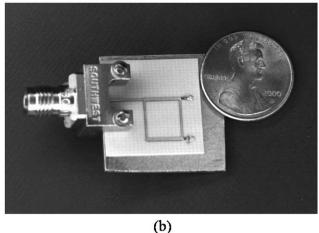
**Figure 1** (a) Schematic of reflection phase shifter with two arms terminated with LC loads for improved tunability. (b) A photograph of the fabricated phase shifter
