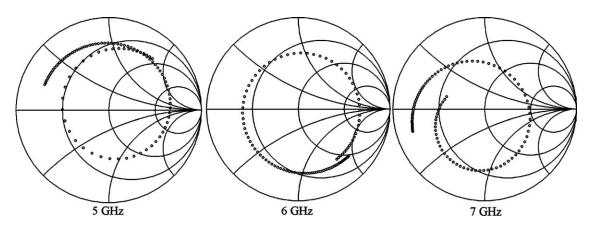
Figure 2 Measured impedance coverage at 5 GHz, 6 GHz, and 7 GHz shows sufficient tuning range
