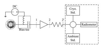
Figure 3 Illustration of the noise-temperature measurement setup. The components in the dashed box represent part of the NIST NFRad system
