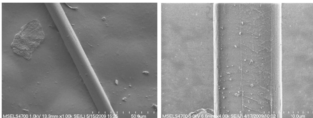
Figure 6: Left: Non-folded virgin PPT fiber. Right: Damage induced by single fold of PPT fiber.
