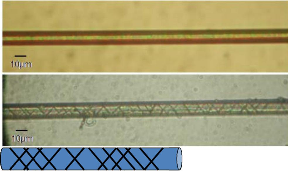
Figure 4: Top fiber: Non-folded virgin PPT fiber. Bottom fiber: Damage induced by single fold of PPT fiber.
