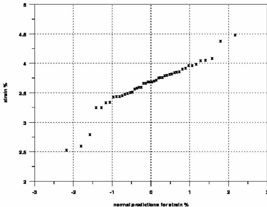
Figure 3: Graphical representation of the non-Gaussian distribution for strain values using Method 1 for the single fold samples. The Y axis represents the sorted experimental strains, the X axis the normal predictions for strain.
