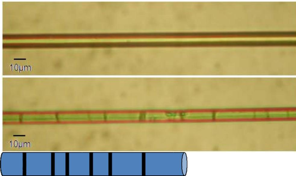
Figure 5: Top fiber: Non-folded virgin PBO fiber. Bottom fiber: Damage induced by single fold of PBO fiber.
