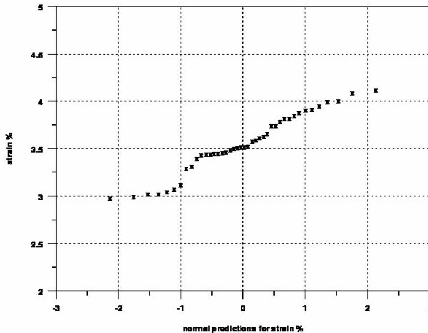
Figure 2: Graphical representation of the non-Gaussian distribution for strain values using Method 2 for the Virgin samples. The Y axis represents the sorted experimental strains, the X axis the normal predictions for strain.
