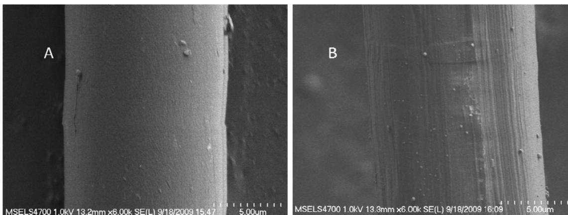
Figure 7: (A) Non-folded virgin PBO fiber. (B) Damage induced by single fold of PBO fiber.
