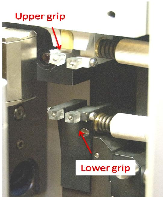
Figure 1. Close-up of the grips used in Method 2.
