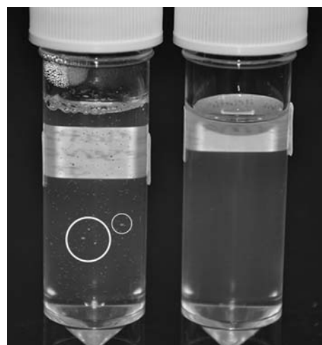
Fig. 9 The vial on the left contains no preservative, and is growing small spots of mold after 20 days. Vial on the right has a volume fraction of 0.12% propionic acid and contains no mold.
