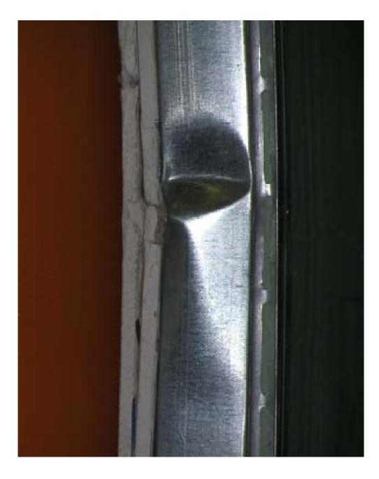
Figure 9 Close-up view of Local Buckling of C-H Stud – Specimen 3
