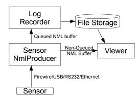
Figure 3: Sensor Subsystem Architecture
