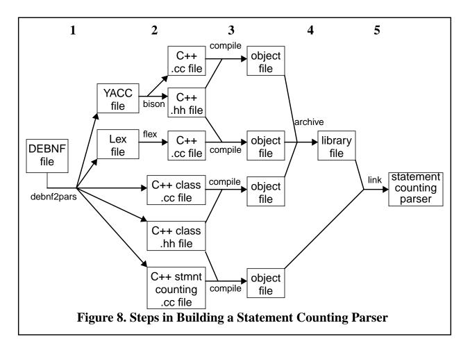
As shown in Figure 8, building a parser starting from a DEBNF file includes the following steps.
