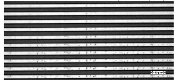
Figure 6. Montage of 10 images during an AC test at 100 Hz of a line fully constrained with SiO<sub>2</sub>. The time series runs from top to bottom. The top image was acquired at 30 s into the test, and the acquisition interval was 10 s. The abrupt change from unvoided to voided is clearly shown.
