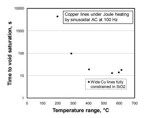
Figure 7. Time interval to void saturation for a series of AC tests of fully constrained wide copper lines tested at 100 Hz, plotted against the cyclic temperature range.
