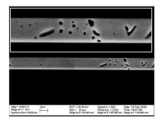
Figure 2. SEM micrograph of a constrained copper line after electrical testing under sinusoidal excitation and removal of the dielectric covering the specimen. This specimen was tested under sinusoidal AC at a peak current density of approximately 14 MA/cm<sup>2</sup>; it self-heated to a temperature of 396 °C and had a lifetime of 1497 s. Note the round and elongated void types. Inset: Expanded display of the right-hand portion of the image
