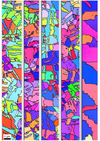
Figure 5. Orientation maps of portions of five damascene copper lines showing the effect of annealing and electrical testing on the grain structure. (a) Grain structure of an as received line. (b) Effect of a 30 h aneal in a vacuum furnace at 300 °C. (c) Orientation map of part of the line shown in Fig. 4 (DC test). (d) Orientation map of a line that received a treatment of 1 h in a vacuum furnace at 420 °C. (e) Orientation map of part of the line shown in Fig. 2 (AC test).
