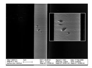
Figure 4. SEM micrograph of a constrained copper line, after electrical testing under DC and removal of the dielectric covering the specimen. It was tested under DC at a current density of approximately 15 MA/cm<sup>2</sup>; it self-heated to a temperature of 413 °C above ambient and had a lifetime of 326 s. Inset: region of specimen with voids. Note the faceted void shapes.
