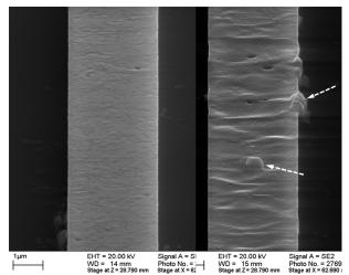
Figure 3. SEM micrograph of copper lines with thin constraint. Left: untested. Right: tested at a peak AC current density of 13 MA/cm<sup>2</sup>. The cyclic temperature range was 262 °C and the lifetime was 2645 s. The prominences near the lower center and upper right in the tested line (arrows) are copper oxide. The bright horizontal contours indicate topographic features (ridges or grooves). Note the voids.
