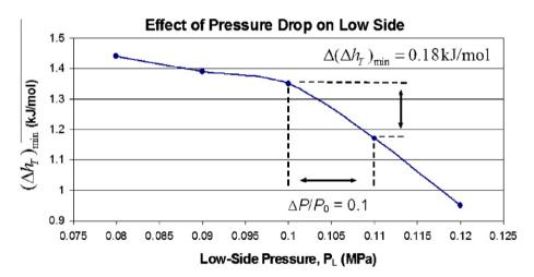
Fig. 4. Effect of pressure drop in the low-side on the minimum enthalpy difference. As shown, a 10% pressure increase on the low-side due to a pressure drop causes 0.18 kJ/ mol loss in enthalpy difference.
