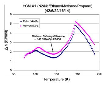
**Fig. 2.** Enthalpy difference vs. temperature of an optimized five-component mixed refrigerant. Both enthalpy difference of 0.1 MPa (1 bar)–1.6 MPa (16 bar) and 0.1 MPa (1 bar)–2.5 MPa (25 bar) are plotted as a function of temperature.
