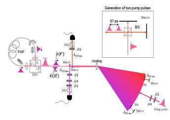
Fig. 9. Schematic for creation of polarization-entangled photon pairs using FWM in a Sagnac interferometer. PBS: polarizing beam splitter. BS: 50/50 non-polarizing beam splitter.  $\lambda/2$  and  $\lambda/4$  are half- and quarter wave plates. Inset is a Michelson interferometer to be inserted into the pump beam path to generate two identical pump pulses for the creation of time-bin entanglement.
