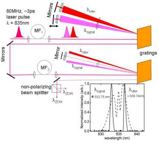
Fig. 7. Schematic for cascaded FWM using two identical pieces of MF to produce frequency-degenerate photon pairs. The inset shows that the dual pump wavelengths incident into the second MF are carved from the broadened spectrum of the laser pulse after propagation in the first MF.
