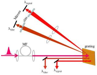
Fig. 5. Schematic for producing photon pairs in MF via FWM and the design of our double-pass spectrometer to spectrally select frequency-correlated signal and idler photon pairs from the broadband output of FWM.
