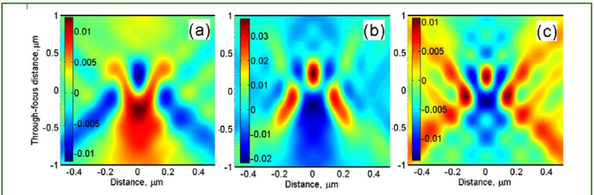
Figure 2. Simulated differential TSOM images obtained for the 2D isolated line target shown in Figure 1(b) for (a) 2.0nm difference in the line width (42nm and 40nm), (b) 2.0nm difference in the line height (82nm and 80nm), and (c) 2.0° difference in the sidewall angle (90° and 88°).
