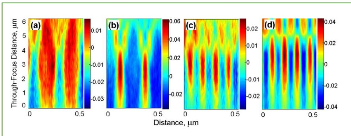
Figure 4. Experimental TSOM images for dense line gratings fabricated with intentional defects. Every tenth line is (a) smaller, or (b) larger by 10nm; or every fifth line is (c) smaller, or (d) larger by 10nm. [ $\lambda = 546\text{nm}$ , nominal line width = 90nm, nominal pitch = 270nm, illumination NA = 0.36, imaging NA = 0.8]
