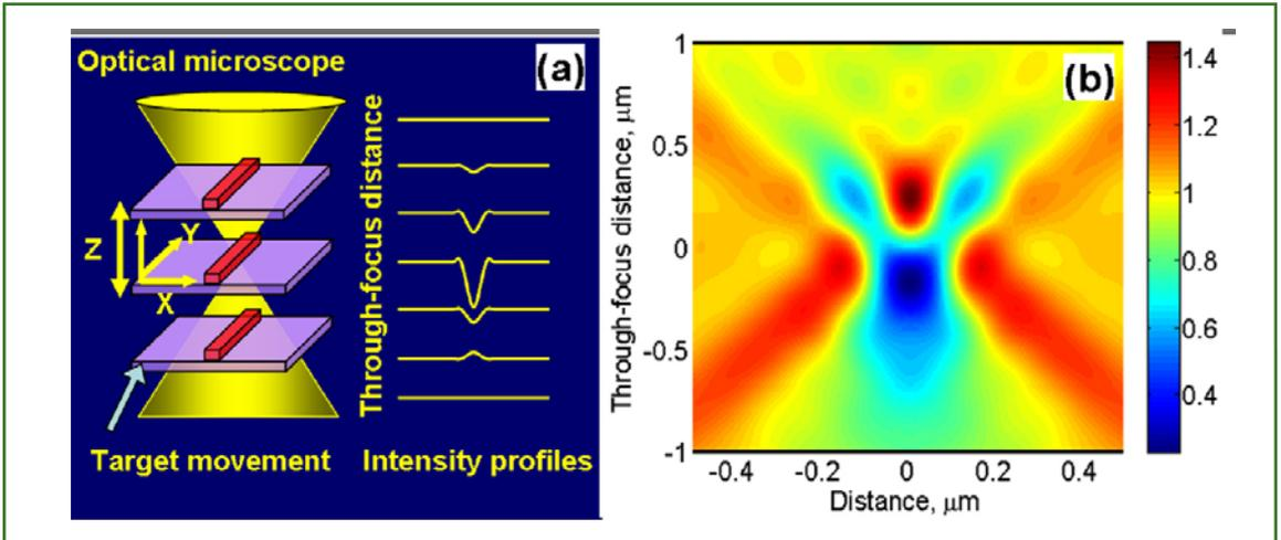
Figure 1. Method to construct a TSOM image. (a) Schematic showing the image-acquisition process by through-focus scanning of an isolated line. The schematic of the cross-sectional image-intensity profiles at the various scan positions is shown on the right side. (b) Simulated two-dimensional TSOM image (X-Z plane) of the isolated line. [Line width = 40nm, line height = 80nm, sidewall angle = 90°,  $\lambda = 193\text{nm}$ , illumination NA = 0.4, imaging NA = 0.95, Si line on Si substrate]
