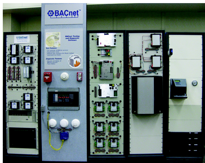
Figure 1 Virtual Cybernetic Building Testbed control hardware. Shown in the photo are the data acquisition unit in the lower left, a range of HVAC control products, a fire detection and alarm system, and on the far right some biometric devices that are part of an access control system. Not shown are other access control devices and a lighting control system.
