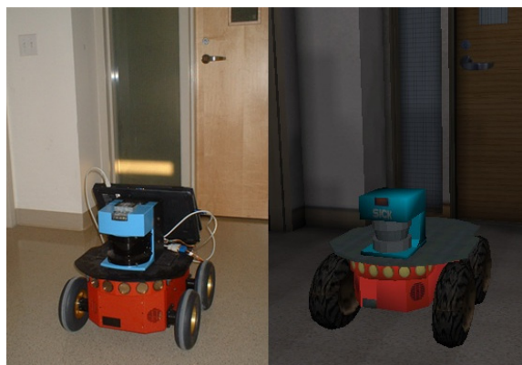
Figure 6: Real and simulated robots observed while validating the range scanner simulation. The cross in Figure 7 shows the position of the robot in the environment, where these pictures were taken.
