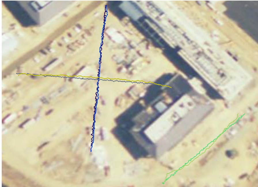
Figure 8: Comparison between the traces produced by the real and simulated GPS sensor. The traces have been superimposed to a satellite image of the University of California, Merced campus.
