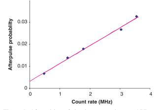
Figure 5. Afterpulsing of the detector under test APD at various count rates. Uncertainty bars are shown. (The color version of this figure is included in the online version of the journal.)
