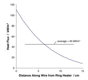
Figure 15. Estimated heat flux along wire in heated conductor test [5].
