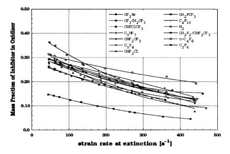
Figure 6. Mass fraction of inhibitor in the oxidizer flow (air) necessary to extinguish a counterflow diffusion flame over heptane, as a function of strain rate ( $T_{air, inlet} = 25$ °C).
