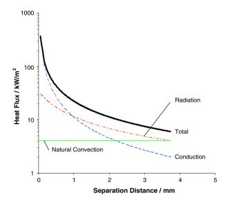
Figure 17. Estimated heat flux from a wire at 922 K (1200°F) to a polymer (at 330°C), as a function of their separation distance.
