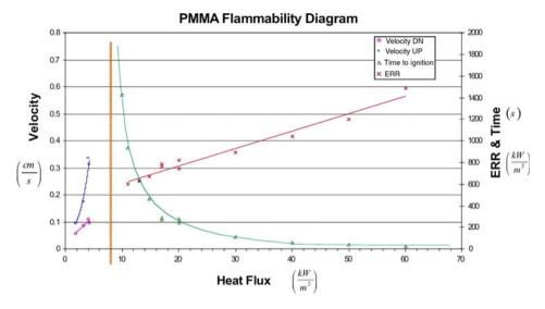
Figure 14. Flammability diagram for PMMA (from Ref. [49]; used with permission of the author).
