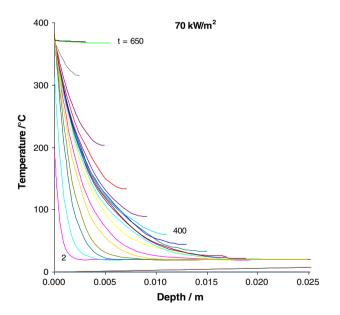
Figure 5. 1-D temperature profile through PMMA slab (initially 25.4 mm thick) as a function of time (indicated on curves), at incident flux or 70 kW/m<sup>2</sup>.
