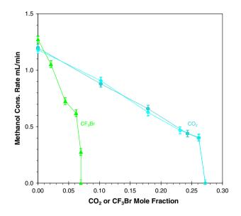
Figure 11. Cup burner methanol consumption rate as a function of  $CO_2$  and  $CF_3Br$  volume fraction in air.
