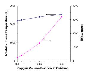
Figure 9. Adiabatic flame temperature and final H-atom volume fraction as a function of oxygen volume fraction in the oxidizer in a  $CH_4/O_2/N_2$  premixed flame.
