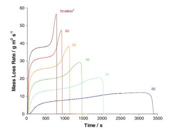
Figure 2. Calculated mass loss rate of 25.4 mm thick PMMA as a function of time for incident external flux rates of (10, 20, 30, 40, 50, 60, and 70)  $kW/m^2$ .
