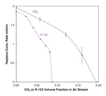
Figure 10. Cup burner heptane consumption rate as a function of  $CO_2$  or R-125 volume fraction in air.
