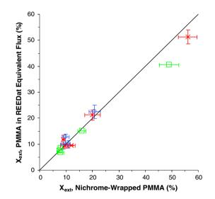
Figure 22. Agent extinguishing volume fraction with the agents in Fig. 21 as well as with IG-541 for PMMA with Nichrome wire heating, or at an equivalent heat flux achieved in the REED device ( $\bigcirc$ : Ref. [57];  $\Box$  and +: 48 W and 192 W cases of Ref. [9].
