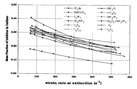
Figure 7. Mass fraction of inhibitor in the oxidizer flow (air) necessary to extinguish a counterflow diffusion flame over heptane, as a function of strain rate ( $T_{air, inlet} = 150^{\circ}$ C).
