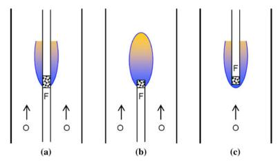
Figure 13. Cylindrical fuel configurations methane-air porous burners (from Ref. [44]; used with permission of the author).
