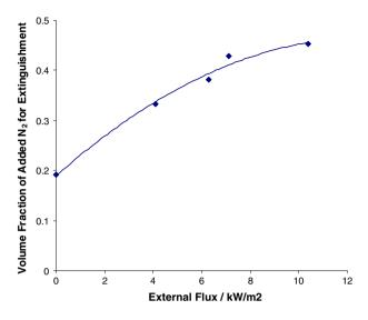
Figure 19. Required nitrogen added to air for extinction of flames over PMMA as a function of external radiant flux [17] (points: experimental data; line: curve fit).
