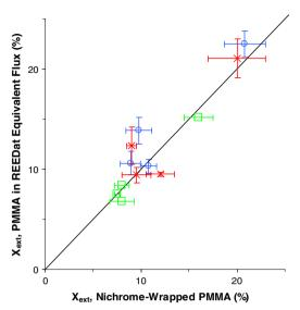
Figure 21. Agent (HFC-23, HFC-227ea, FC-2-1-8, and FC-3-1-10) extinguishing volume fraction for PMMA with Nichrome wire heating, or at an equivalent heat flux achieved in the REED device ( $\bigcirc$ : Ref. [57];  $\Box$  and +: 48 W and 192 W cases of Ref. [9].
