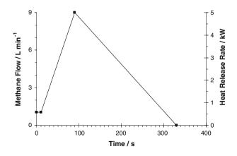
Figure 20. Input power versus time for NEBS fire test [71].
