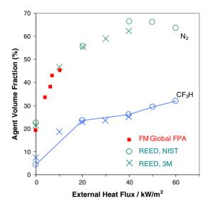
Figure 23. HFC-23 or  $N_2$  volume fraction for extinguishment of PMMA in the REED device as a function of external heat flux (NIST and 3M results are given). Tests with  $N_2$  extinguishing PMMA in the FM Global FPA [17] are also shown.
