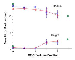
Figure 12. Flame height and radius for methane-air cup-burner flames with  $CF_3Br$  added to the air stream at increasing volume fraction [44].
