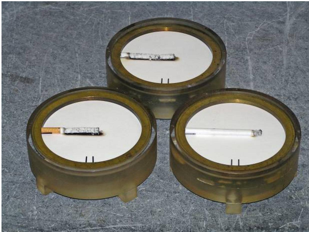
**Figure 2. Photograph of Typical Results of Determinations using ASTM E2187-04. Top: full-length burn of the CTC (a non-filter cigarette); Left: full-length burn of a filter tip cigarette; Right: ceased burning of a low ignition strength cigarette.**
