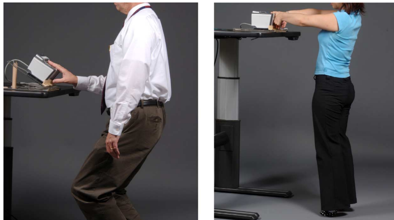
Fig. 6. Left: A taller participant presents to a sensor at a 30 degree angle on a 39 in high counter. Right—A shorter participant presents to a flat sensor on a 49 in high counter. Note that the shorter participant cannot keep their feet flat on the ground.
