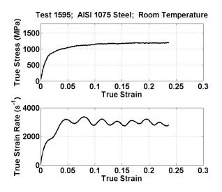
Figure 3: Results of Kolsky bar test on roomtemperature sample of AISI 1075 steel. True stress at 10 % true strain is approximately 1140 MPa; true strain rate is approximately 3500 s<sup>-1</sup>.
