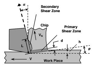
Figure 1: Schematic illustration of orthogonal cutting.
