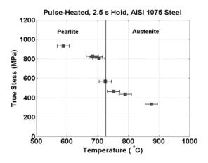
Figure 4: Kolsky bar experimental data on AISI 1075 steel; pearlitic room-temperature samples were pulse-heated and then held at temperature for 2.5 s; vertical line denotes the eutectoid temperature (723 °C); squares denote the flow stress at 10 % true strain; error bars denote  $2\sigma$  [11].
