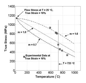
Figure 5: Flow stress at 10 % true strain. Upper (dash-dot) curve: m=1.6; middle (solid) curve: m=1.0; lower (dash) curve: m=0.7. Vertical line denotes eutectoid temperature. Circle is experimental data from room temperature test; squares are experimental data from tests in which the sample was pulse-heated and then held at constant temperature for 2.5 s before impact.
