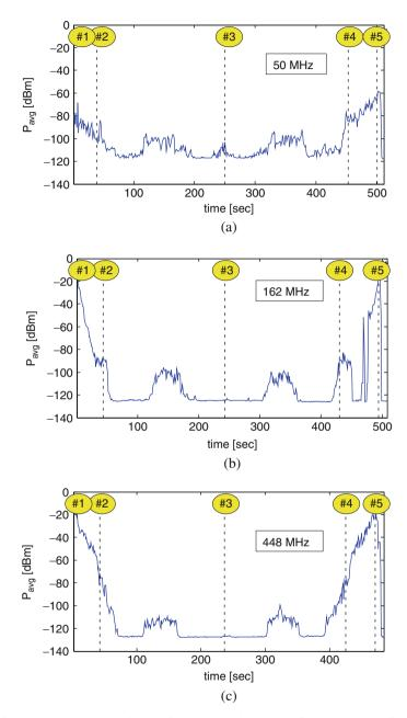
Fig. 9.6 Received-power data in the Greathouse Mine tunnel for three carrier frequencies: (a) 50 MHz, (b) 162 MHz, (c) 448 MHz. In each case the #2 and #4 vertical *dashed lines* correspond to the turn at 100 m: once on the way into the tunnel and once on the way out. The #3 *dashed line* represents the end point. For the Greathouse mine tunnel, the end point was approximately 350 m into the tunnel, as shown in Fig. 9.4(b)
