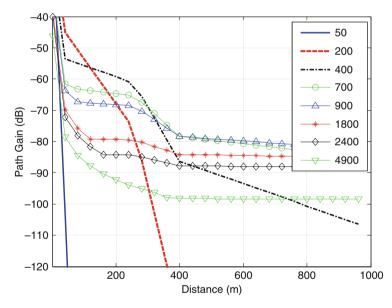
**Fig. 9.16** Path gain calculated for the 6 m  $\times$  4.5 m subway tunnel shown in Fig. 9.15 for eight different frequencies (in MHz). Three distinct propagation regions can be identified: Line-of-sight (less than 200 m), large-radius curve (200–400 m), and a straight, non-line-of-sight section (greater than 400 m) [15]
