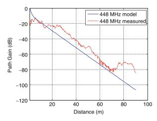
**Fig. 9.11** Comparison of measured and modeled data for the Hazel-Atlas tunnel. The carrier frequency is 448 MHz. The modeled data simulate waveguide propagation for a waveguide whose physical parameters approximate those of the tunnels
