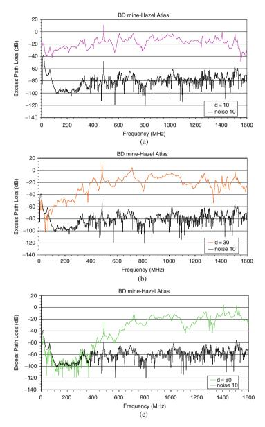
**Fig. 9.8** Excess path loss measurements from 25 MHz to 1.6 GHz carried out at different distances: (**a**) 10 m, (**b**) 30 m, and (**c**) 80 m from the portal of the Hazel-Atlas mine tunnel. The "noise" curves were measurements taken with no transmitted signal. These were not made at every location, and are presented to give an indication of the dynamic range of each measurement (received signal power relative to noise power)
