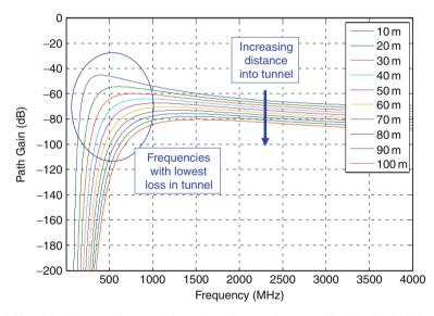
**Fig. 9.12** Path gain versus frequency for various distances in a tunnel having physical characteristics similar to those of the Hazel-Atlas tunnel. Frequencies of approximately 400 MHz–1 GHz propagate further than either lower or higher carrier frequencies
