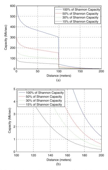
Fig. 9.14 Channel capacity predicted by the Shannon theorem for a carrier frequency of 2.4 GHz and a modulation bandwidth of 20 MHz. At 160 m, where we experienced intermittent video, 15% of the Shannon limit is  $\sim$ 1 Mb/s, which is the minimum data rate specified for an 802.11b signal before it fails
