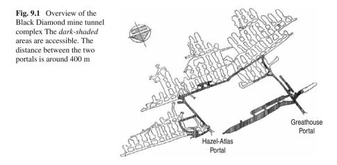
The cross-sectional dimensions of the Hazel-Atlas tunnel varied from approximately 1.9 m (6', 3'')  $\times$  1.9 m to as much as 2.6 m (8', 5'')  $\times$  2.4 m (8', 0''). The dimensions of the Greathouse tunnel were somewhat bigger, up to approximately 3 m square in places. The Hazel-Atlas tunnel contained railroad tracks spaced 61 cm (24") apart. Both tunnels consisted of a straight section followed by a 90° turn around a corner, as shown in Fig. 9.1.
