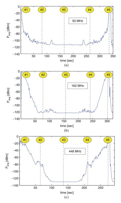
**Fig. 9.5** Received-power data in the Hazel-Atlas Mine for three carrier frequencies: (**a**) 50 MHz, (**b**) 162 MHz, (**c**) 448 MHz. In each case the #2 and #4 vertical *dashed lines* correspond to the turn at 100 m: once on the way into the tunnel and once on the way out. The #3 *dashed line* represents the end point. For the Hazel-Atlas mine tunnel, the end was at 200 m, shown in Fig. 9.4(a)
