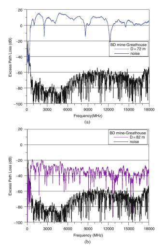
Fig. 9.9 Excess path loss for frequencies from 1 to 18 GHz in the Greathouse tunnel (a)72 m into the tunnel in a line-of-sight condition, and (d) 82 m into the tunnel in a non-line-of-sight condition
