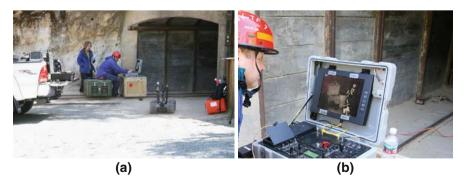
**Fig. 9.10** (a) Robot operator positioned at the entrance to the Hazel-Atlas mine tunnel. (b) The robot was operated in a non-line-of-sight condition more than 100 m inside the tunnel
