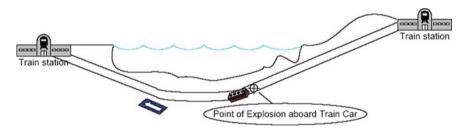
**Fig. 9.15** Representative tunnel environment consisting of a 1500 m smooth-walled underground tunnel with a large-radius curve. An environment such as this could be specified for the development of test methods to evaluate the performance of robots for US&R applications (drawing not to scale)
