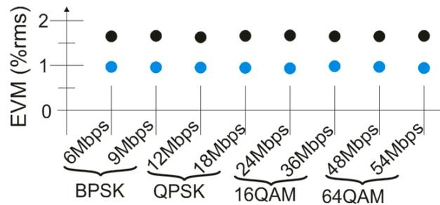
Fig. 2: EVM for the modulation types used in the 802.11a Standard for a low-distortion case (blue) and a medium-distortion case (black).
