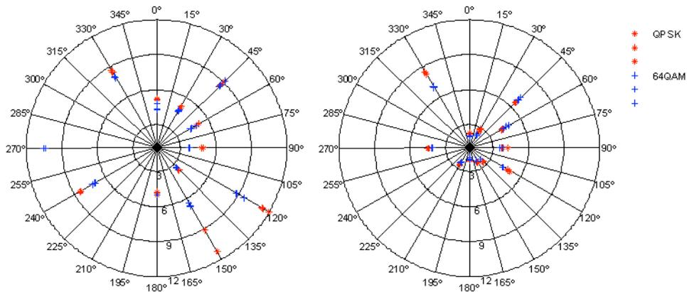
Fig. 5: Rx position M2 (closest to tunnel) EVM results for QPSK and 64QAM at 2.412 GHz and 4.95 GHz. The radial scale is percent EVM.
