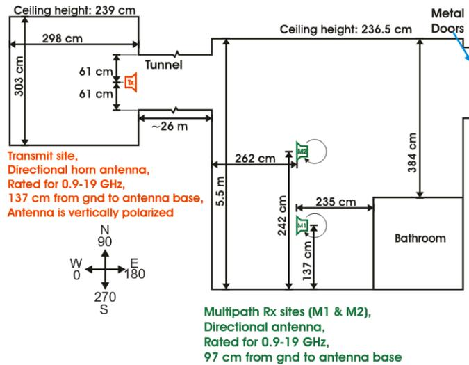
Fig. 3: Diagram of multipath environment for multipath measurements.
