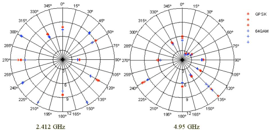
Fig. 4: Rx position M1 (closest to wall) EVM results for QPSK and 64QAM at 2.412 GHz and 4.95 GHz. The radial scale is percent EVM.
