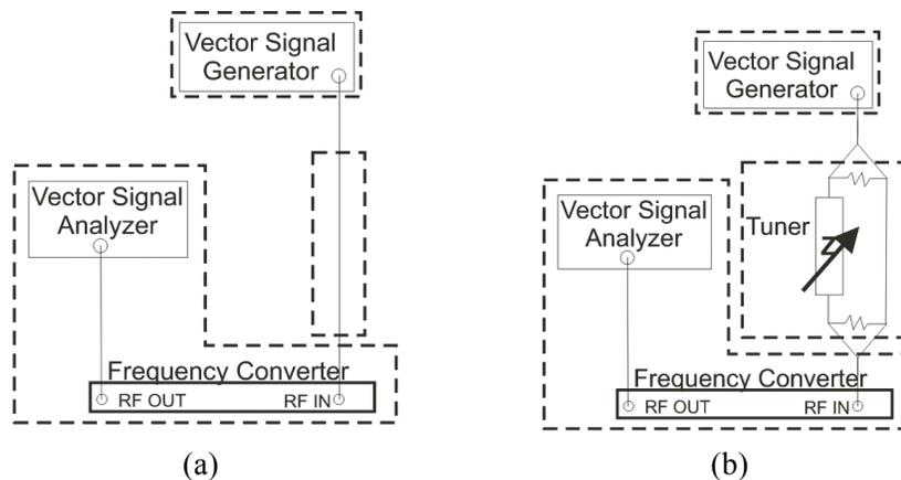
Fig. 1: Lab setup for low-distortion (left) and medium-distortion (right) cases.
