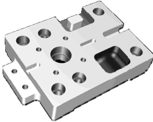
Figure 3.4. Some Stereotypical Features: holes, pockets, slots, planar faces, steps, bosses and freeform surfaces.
