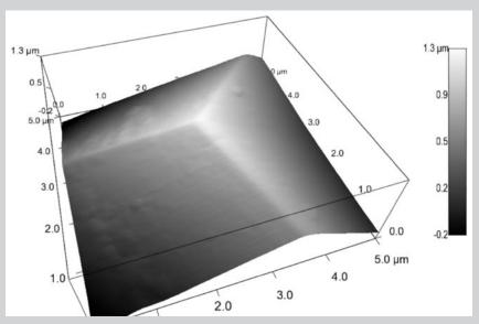
Figure 3. A scanning probe microscopy image of the probe used to carry out the indentations shown in Figure 2. This three-sided Berkovich geometry shows the tip rounding that is unavoidable during manufacture.
