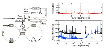
Fig. 1: Left: schematic of the comb (the CEO locking branch is not shown); BPD: balanced photodetector, ISO: isolator. Right: normalized spectrum (shifted by -50 MHz, top) as well as phase ( $S_{\varphi}$ ) and amplitude ( $S_A$ ) noise power spectral density (PSD) (bottom) of the optical lock beat
