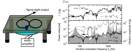
Fig. 2: Left: schematic of the shaking experiment. The laser actually covers the complete breadboard surface. Right: phase noise of the optical and CEO locks under vibration and average vibration amplitude on the breadboard (bottom); vibration sensitivity  $\Gamma$  of the optical lock (top).
