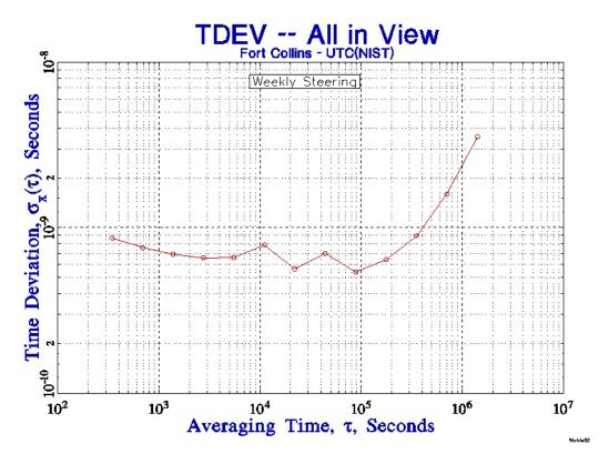
Figure 10. The time deviation of the difference (Fort Collins – Boulder) using weekly steering.
