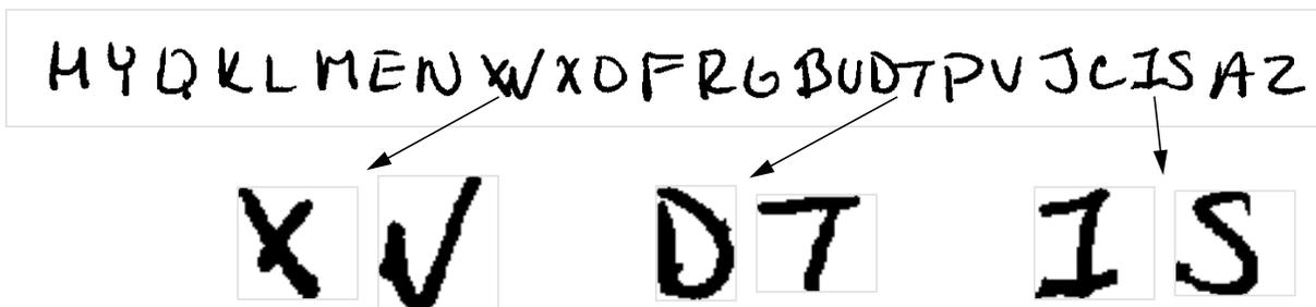
Figure 9. Segmentor results of splitting components apart.
