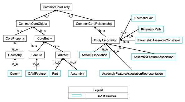
Figure 3: Open Assembly Model, OWL version (highlighting is-a relationship)
