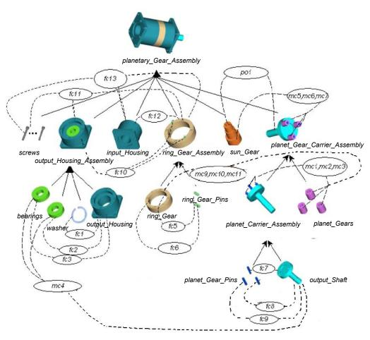
Figure 10: Case study: planetary gear system
