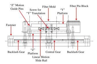
Fig. 2 Side view of fiber-setting device with gear assembly
