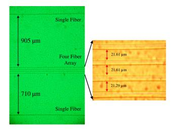
Fig. 6 Typical 2-D combinatorial microcomposite
