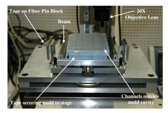
Fig. 4 Fiber-setting device on MM-40 measurescope stage
