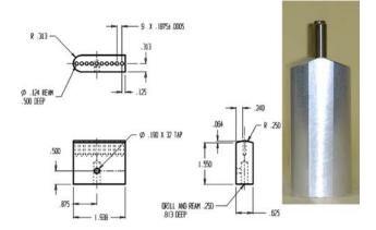
Fig. 3 Schematics of fiber pin block. Inset shows triangular surfacing away from fiber pins; this modification helps maintain array uniformity at small inter-fiber spacings
