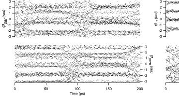
Figure 2(a). Phase eye patterns (2 bit length) as measured by the two orthogonal demodulators.channels (clearly not polarization-aligned with the POLMUX channels).
