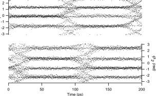
**Figure 2(b)**. Phase eye patterns of the two orthogonal polarization states aligned with the POLMUX axes. Recovered with a software rotation of  $\theta$ =150.305°. The time shift between  $\varphi_{par}$  and  $\varphi_{perp}$  is real and a consequence of the delay difference in the POLMUX arms.
