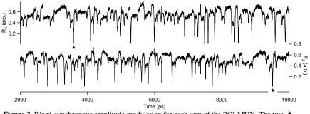
**Figure 3.** Word-synchronous amplitude modulation for each arm of the POLMUX. The two  $\blacktriangle$  symbols indicate an equivalent point in each pattern. The delay between these points (5.9 ns) is the delay between the POLMUX arms.
