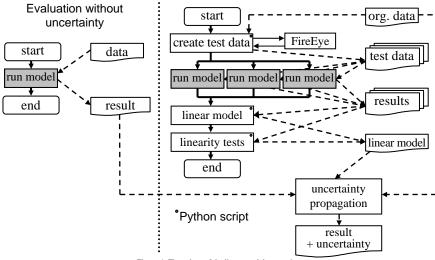
Figure 4: Flow chart of the linear model generation
