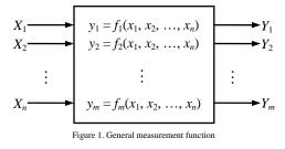
The GUM method can be applied to any kind of calculation scheme where we assume that we calculate some number m of results  $Y_k$  based on n input quantities  $X_i$  and therefore m functions  $f_k$  exist which link the input to the output (see Figure 1). Fortunately we do not need to know the functions in detail. To employ the GUM method it is enough if we know a linear equivalent of the functions around the value of the input quantities.
