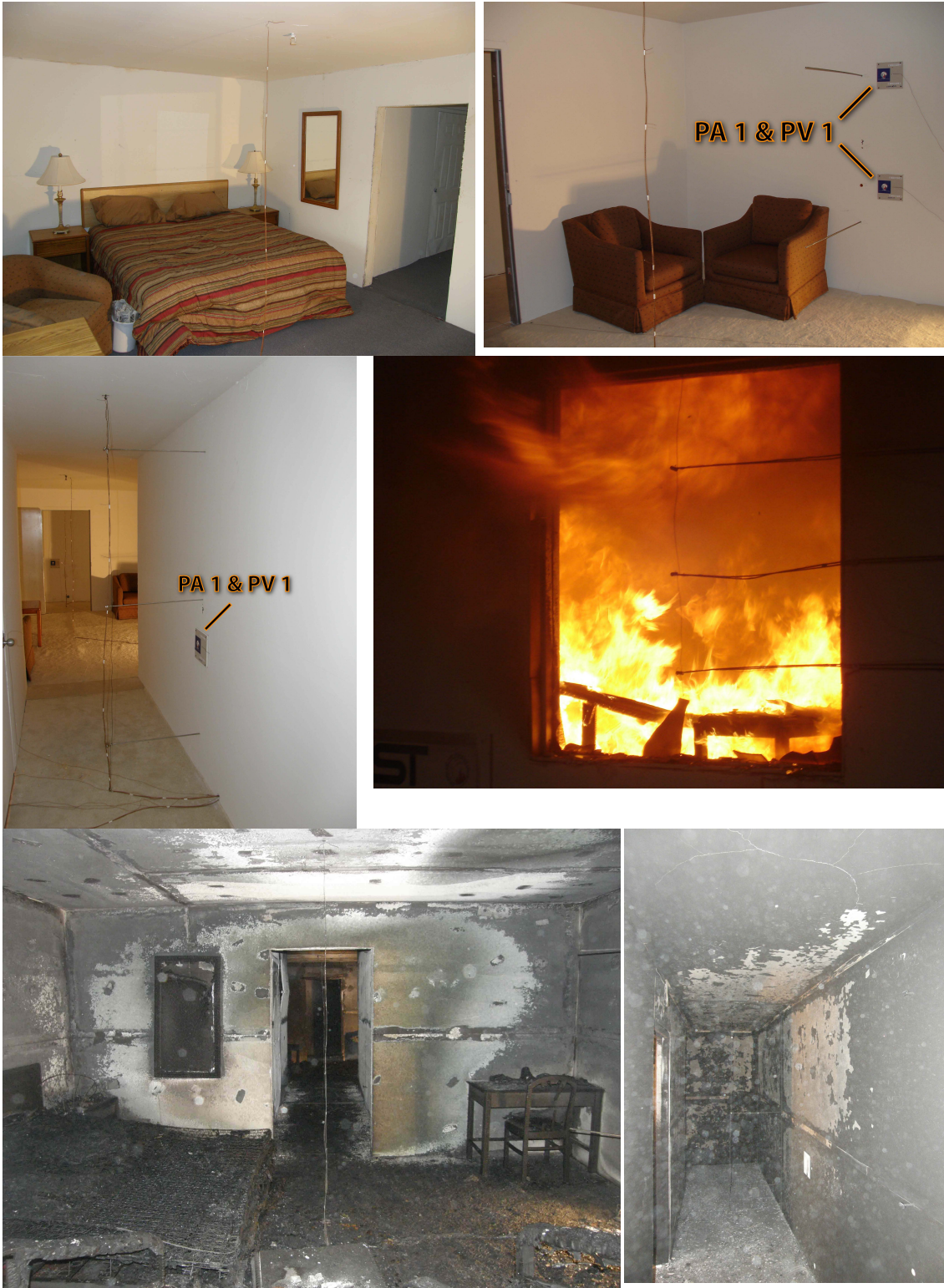
Figure 3-5. Photographs show the bedroom (top left), the living room (top right), the center hallway (center left) before the test; the fire in the bedroom (center right), the bedroom (lower left) and the end corridor (lower right) after the fire test. Tags PA 1 and PV 1 are shown in Figure 3-1 and Figure 3-2.
