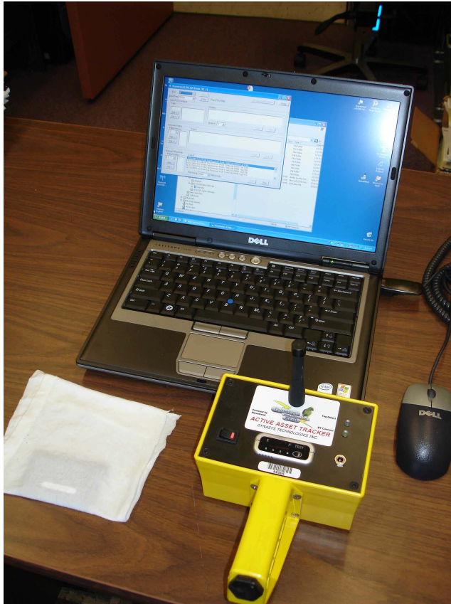
Figure 4-5. Photograph showing the complete active RFID reader system and one of the wet test specimens.
