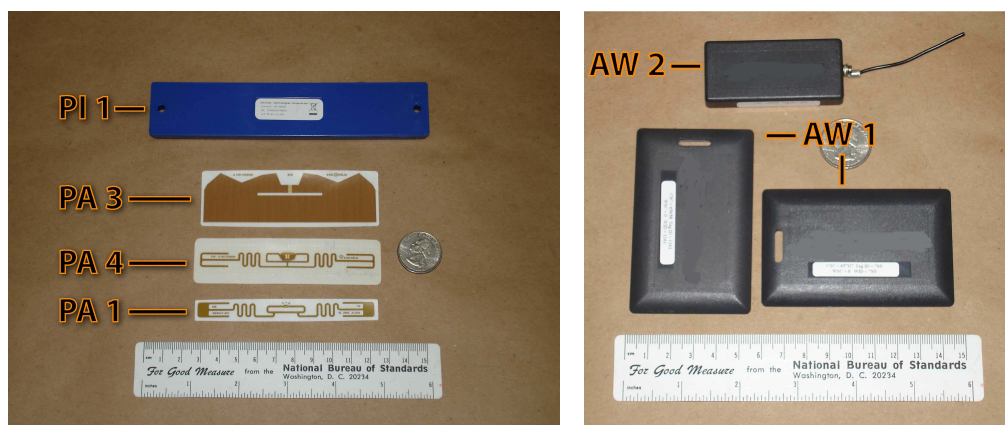
Figure 1-1. Photographs showing examples of passive tags (left) and active tags (right) with no instrumentation.
