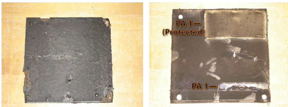
Figure 3-6. Photographs showing passive RFID tag after fire exposure, the tags on the left specimen board had burned away.
