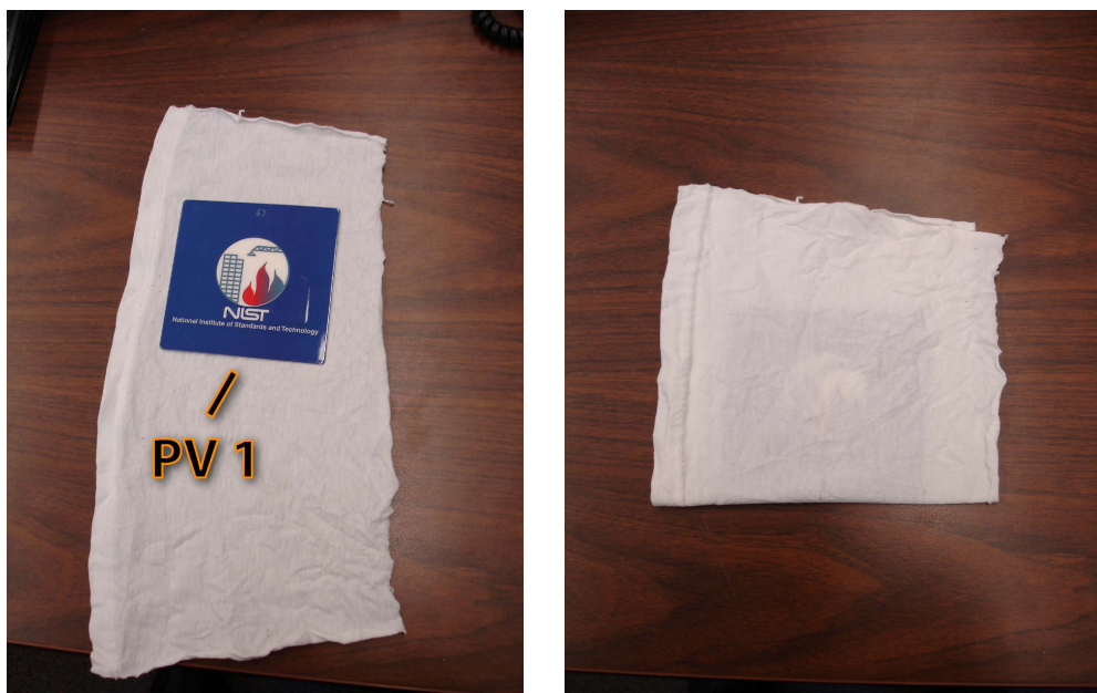
Figure 4-3. RFID tag (PV1) encapsulated in plastic with T-shirt fabric (left); RFID tag enclosed in dry T-shirt fabric (right).
