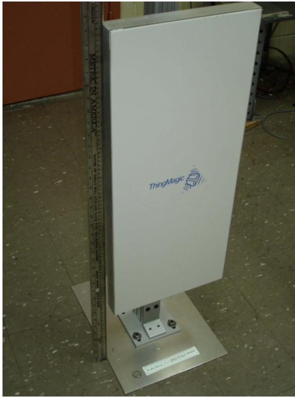
Figure 4-1. Passive RFID tag reader antenna used for wet fabric study.
