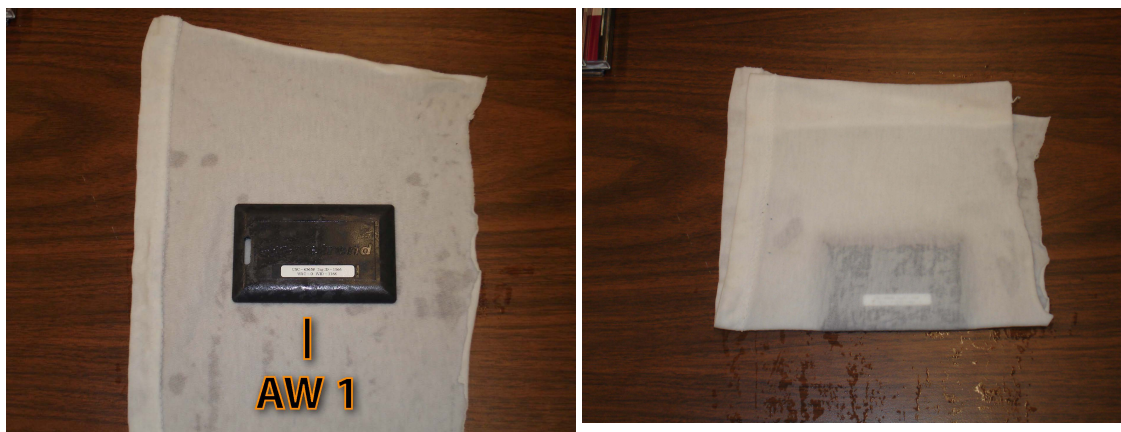
Figure 4-4. Active RFID tag (AW1) with T-shirt fabric (left) and RFID tag enclosed in wet T-shirt fabric (right).
