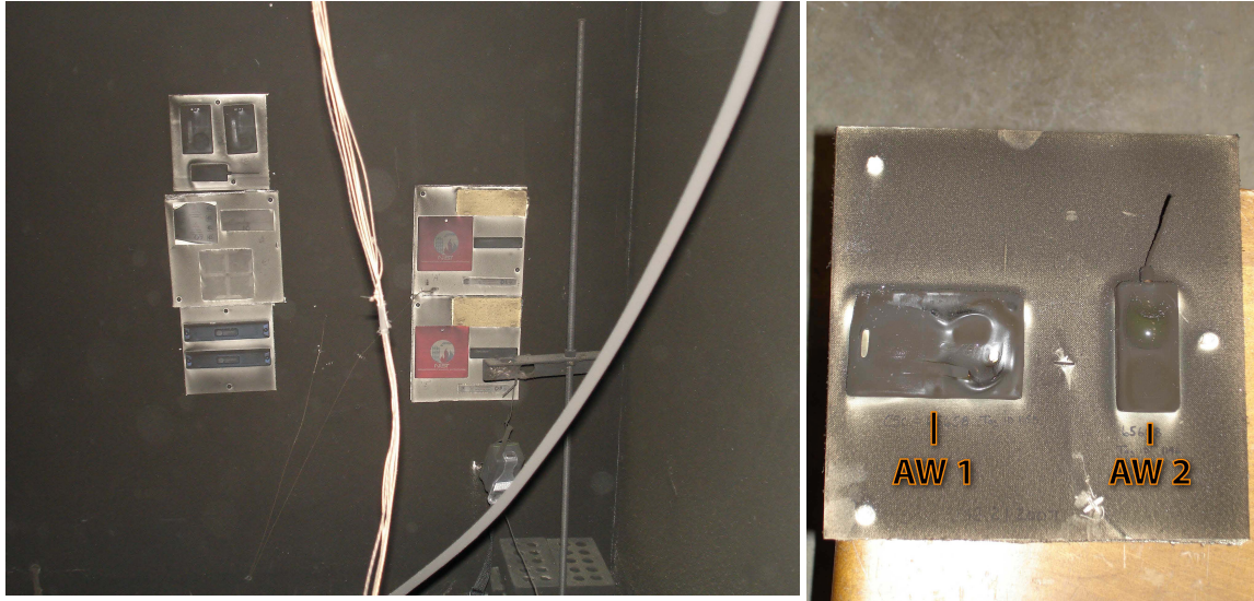
Figure 3-13. Photographs showing fire test damage to passive and active RFID tags. Note: RFID tag identification for these photos is found in Figure 3-1 and Figure 3-2.
