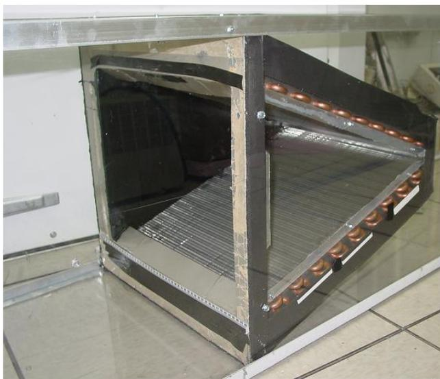
Figure 6. A-Shaped Coil Test Section
