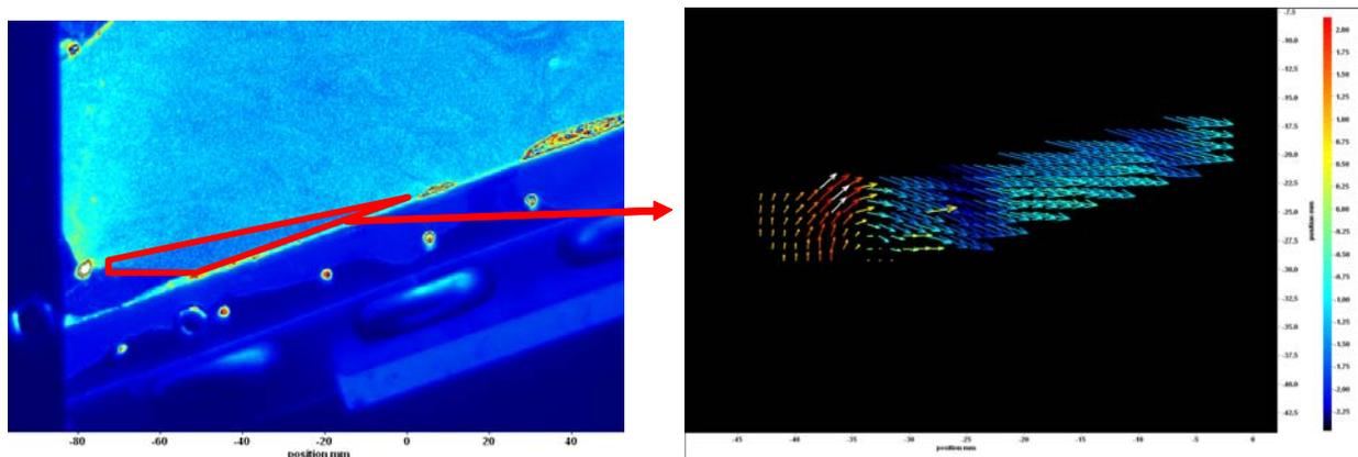
Figure 7. PIV Measurement showing A-Coil Recirculation Zone
