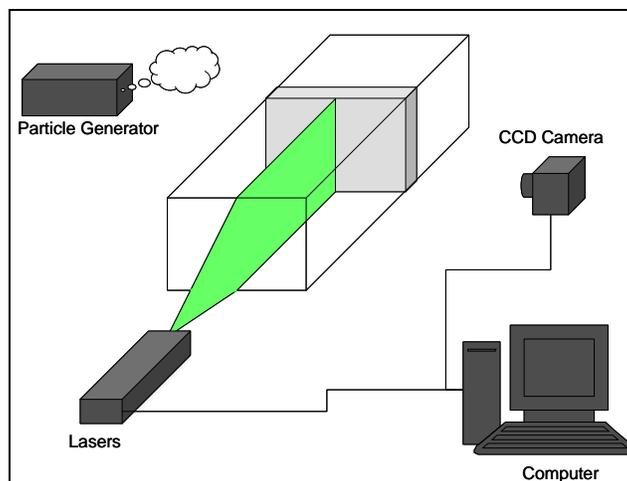
Figure 2. PIV Measurement Apparatus
