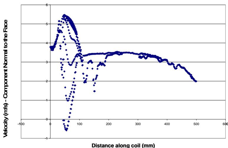
Figure 8. One-Dimensional Air Velocity at the Inlet to the A-Coil– 190 mm
