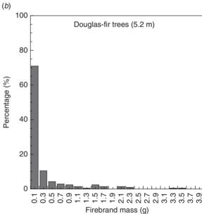
**Fig. 4.** (a) Mass distribution of collected firebrands for 2.6-m Douglas-fir trees. (b) Mass distribution of collected firebrands for 5.2-m Douglas-fir trees
