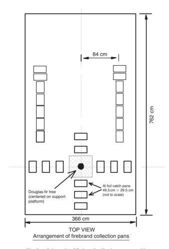
Fig. 2. Schematic of firebrand collection pan assembly.
