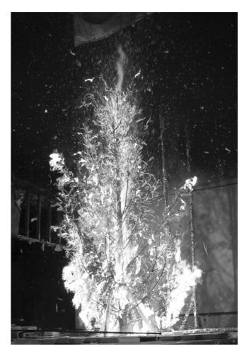
Fig. 1. Photograph of a burning Douglas-fir tree (5.2 m) used for firebrand collection.
