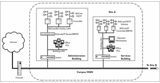
Figure 2: Campus network with facility networks using campus WAN for high-level BACnet communications.
