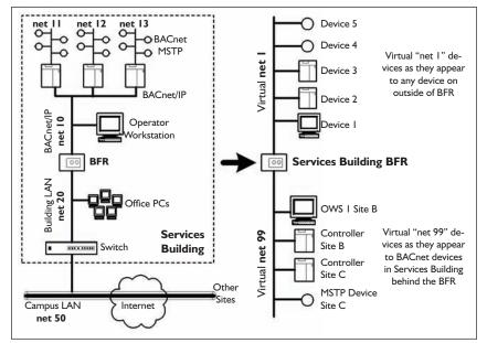
Figure 3: The services building, now with BFR in place, shows the different physical networks (left) and the translated "virtual" networks (right).
