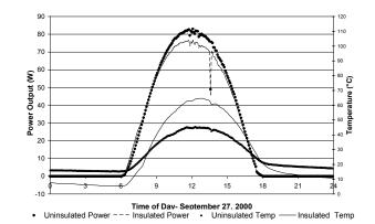
Figure 3 Single Crystalline Power Output and Temperature: Uninsulated Versus Insulated
