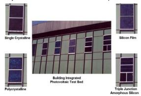
Figure 1 Photovoltaic BIPV Test Bed
