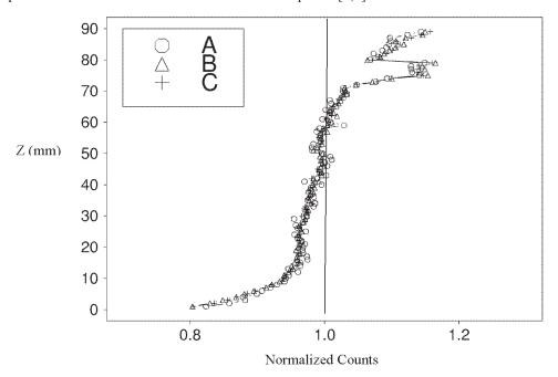
**Fig. 7.** Normalized counts from the vertical scans of a paste specimen in experiment *IVP* for three different intensities (*A, B,* and *C*). See Table 1 for more details. The profiles were determined by averaging the points at each level from 20 scans.
