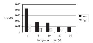
Fig. 3. Normalized Root Mean Square Errors (*NRMSE*) as a function of integration time for experiment *WVP* at low (30 kV; 200  $\mu$ A;  $\approx$ 850 counts per second) and high (35 kV; 700  $\mu$ A;  $\approx$ 12 000 counts per second) x-ray source intensities. The data from the 30 s integration time at the high intensity was used as the true profile for the calculation of the *NRMSE*. See Table 1 for more information on experiment *WVP*.
