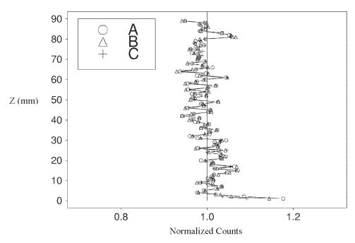
**Fig. 8.** Normalized counts from the vertical scans of a mortar specimen in experiment *IVP* for three different intensities (*A, B,* and *C*). See Table 1 for more details. The profiles were determined by averaging the points at each level from 20 scans.
