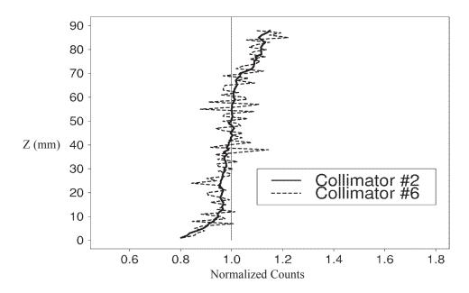
**Fig. 5.** Normalized counts for the paste specimen in experiment *CVP*. The data were taken from vertical profiles with collimator #2 and collimator #6. See Table 1 for more information about experiment *CVP* and Table 2 for more information about the collimators.
