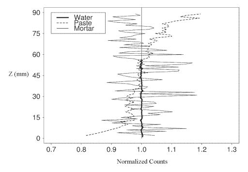
**Fig. 2.** Vertical profiles of normalized counts for water, paste, and mortar specimens from experiment *IVP*. Each mean profile was determined by averaging together four vertical scans at one horizontal location.
