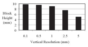
**Fig. 12.** Estimates of the epoxy block height based on the count data from experiment *WEVP*. The actual height of the block is 10 mm.
