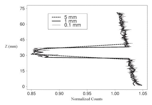
**Fig. 11.** Normalized Counts from the *WEVP* experiments in which a water-filled cuvette with an epoxy block placed inside the cuvette near its middle was sampled.
