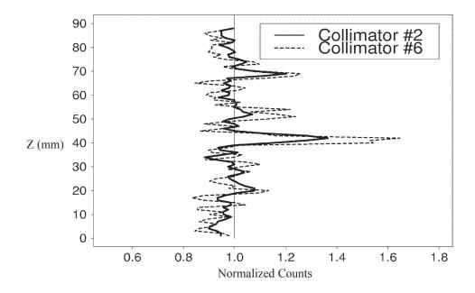
**Fig. 6.** Normalized counts for the mortar specimen in experiment *CVP*. The data were taken from vertical profiles with collimator #2 and collimator #6. See Table 1 for more information about experiment CVP and Table 2 for more information about the collimators.
